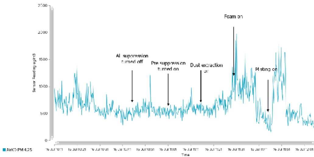
Tests on different systems on and off takes place
