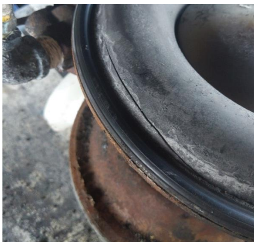
Figure 4. Example of diaphragm failure due to fatigue
