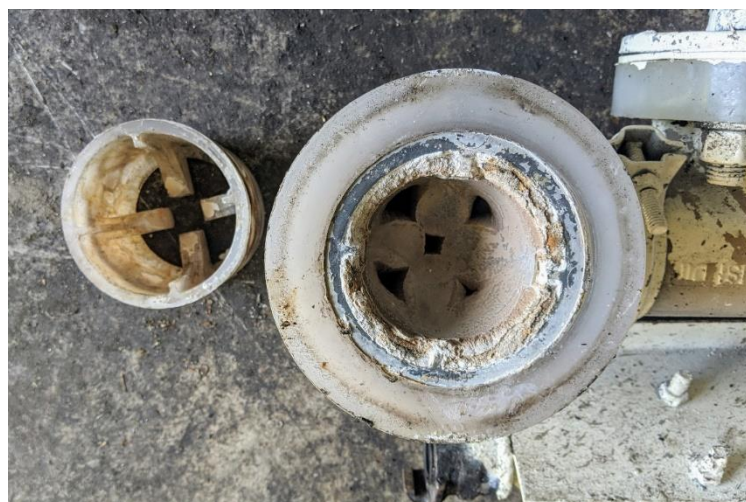
Figure 1. Calcification of pump after 498 days in service
