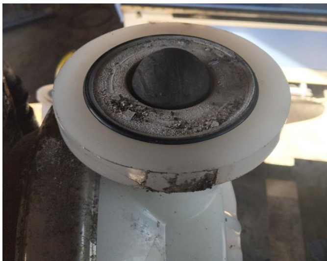
Figure 6. Example of pump failure due to valve seat wear
