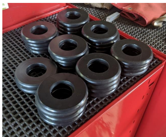
Figure 8. Valve seats made from nylon
