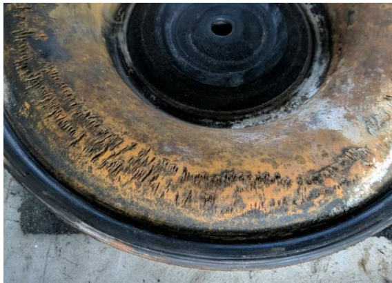
Figure 5. Example of diaphragm failure due to abrasion
